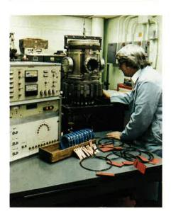
This high vacuum heat treating bell jar determines the effect of atmosphere and temperature during the annealing of different grades of tungsten wire as well as evaluating its thermal stability and recrystallized structures.
