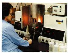
The elevated temperature strength properties are measured to better understand the response of wire to varying application conditions. Wire is normally tested in hydrogen although it can be measured in either vacuum or inert atmospheres.
