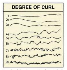
In determining degree of curl, a two-foot length of wire is allowed to hang in a 1" catenary. It is then compared to this chart and rated accordingly.
