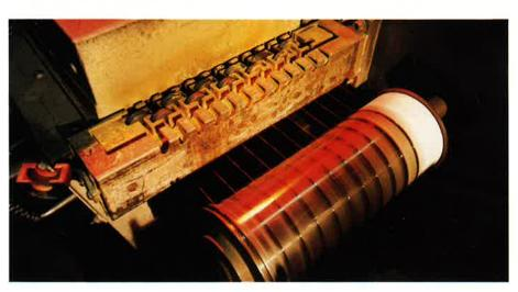
Multiple die equipment in which temperature, drawing speed, and die geometry are carefully controlled, is used to produce very small diameter tungten wire.
